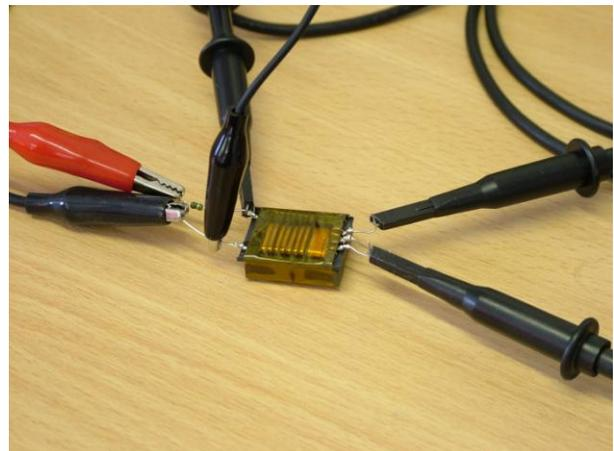
Above shows the transformer being subjected to testing and for all the tests the same probes and connections were used to complete the measurements. Therefore, as minimal alterations were necessary, only the addition of Loss load and longitudinal resistors added, all the tests were completed without the need for sophisticated fixtures.
