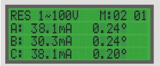
Figure 3. Excitation current results with single-phase test
